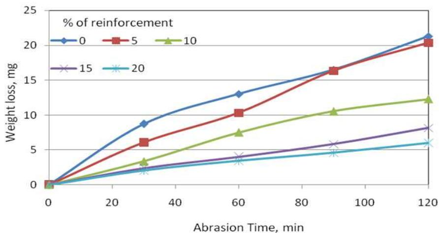
Figure 4: Average Wear Rate as a Function Wear Duration for Al/TiC Composites Abraded by Alumina Slurry for Different Size of Particles
