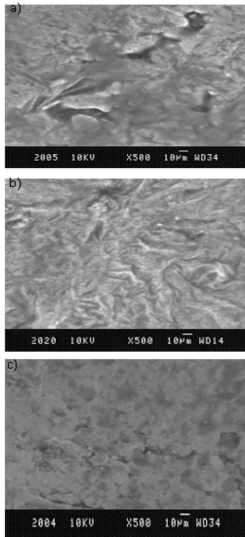
**Figure 7: Worn-Out Surface Ball-Crater Morphology of (a) Al 6061 Alloy, (b) Al/5 % Tic and (c) 20% Tic Samples Abraded by the Aluminum Slurry**
