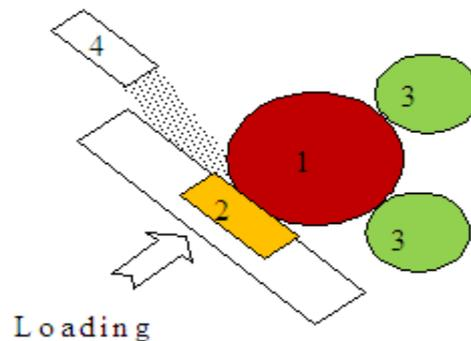
**Figure 2: Ball-Cratering Tribometer Schematic Diagram**
