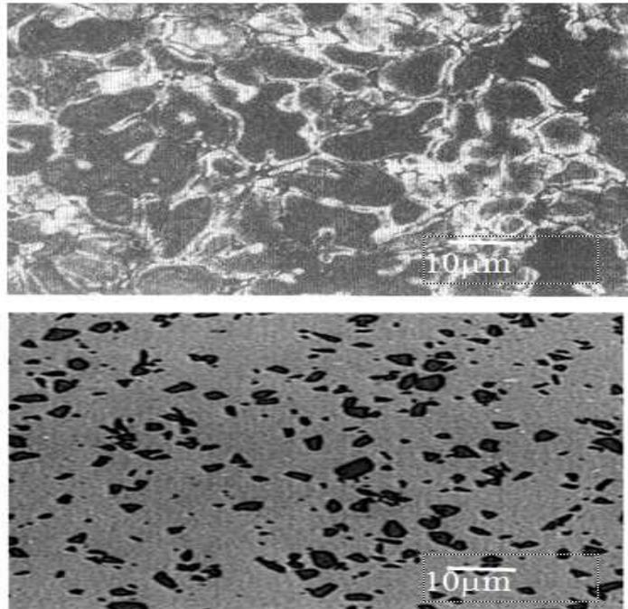
Figure 3: Microstructure of a) Etched Al and b) Unetched Al / 20% TiC Composites
