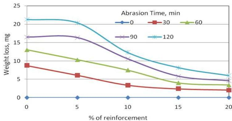
**Figure 6: Variation of Mass Loss with % of Reinforcement for Al/TiB<sub>2</sub> Composites Abraded by Alumina Slurry for Different Sliding Duration**
