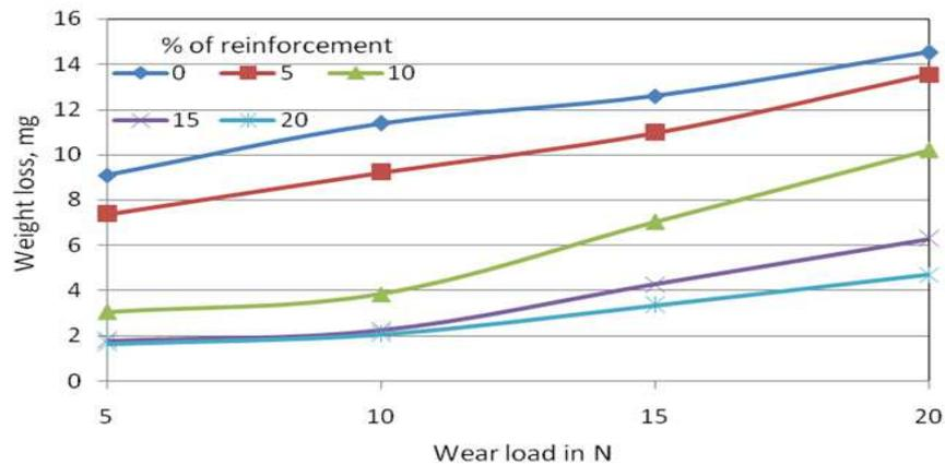
**Figure 5: Variation of Mass Loss with Normal Load for Al/TiC Composites Abraded by Alumina Slurry for Different Sliding Time Min**
