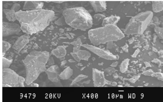
**Figure 1: Al<sub>2</sub>O<sub>3</sub> Abrasive Particles of 90–150 µm size**
